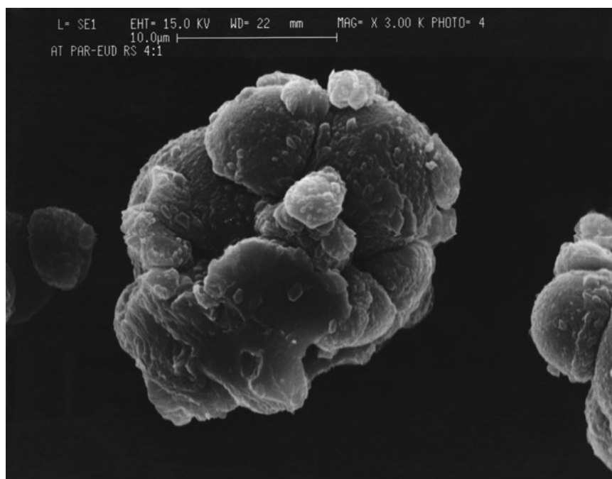
Figure 4. SEM image of paracetamol/eudragit RS 4:1 microspheres.
